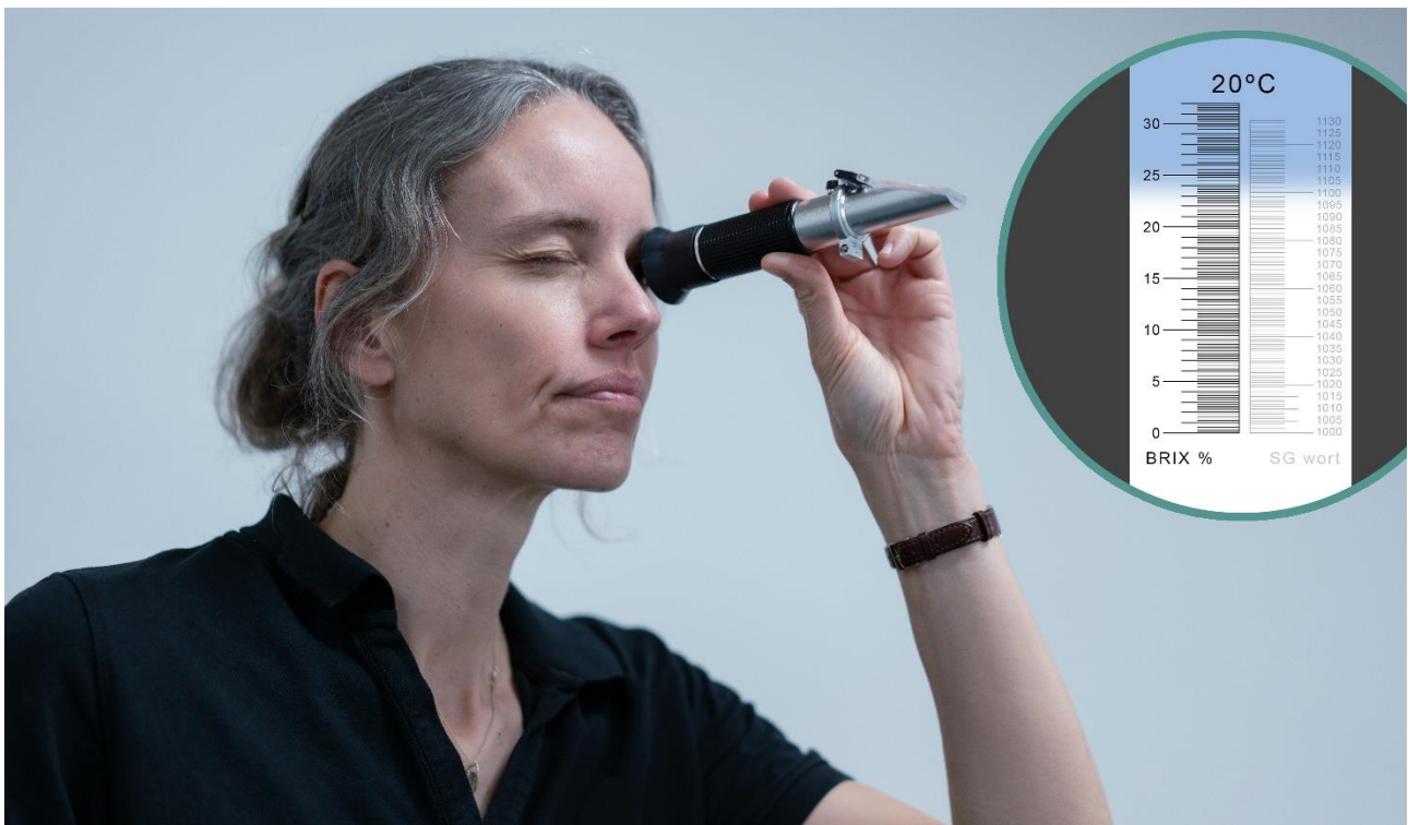
Figure 2: We recommend testing colostrum quality using a BRIX refractometer, to ensure that all calves receive high quality colostrum.
